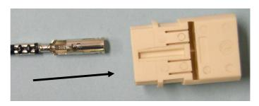
• Orientation of the tab of the coax with the slot of the housing.
